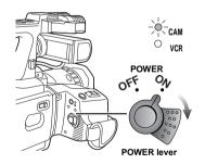
Turn the POWER lever to the ON position. The CAM (red) lamp lights, and the camera-recorder switches to shooting pause mode.
